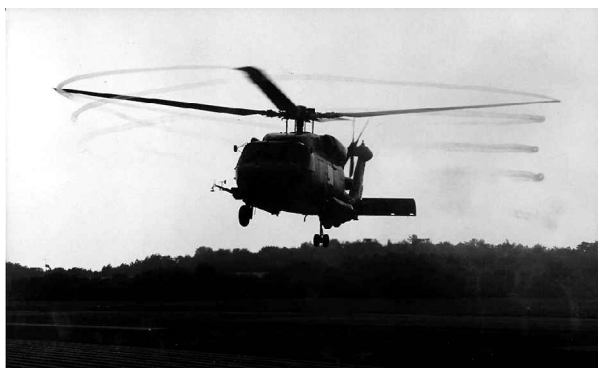
Fig. 4 Natural condensation inside the tip vortices generated by a hovering helicopter.
